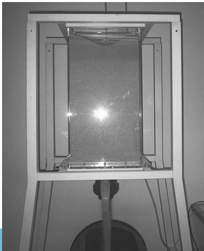
Figure 1: The small-scale silo provided with a flat bottom (0.8m x 0.4m x 0.25m)
