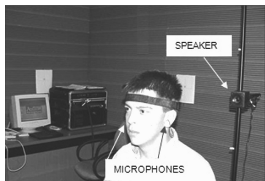
Fig. 1 Empirical HRIR measurement at FIU.
